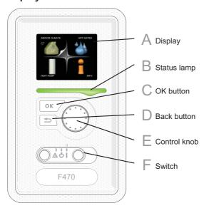
There is a display unit behind the heat pump door, which is used to communicate with F470. Here you:
