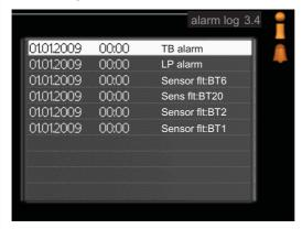
To facilitate fault-finding the heat pump operating status at alarm alerts is stored here. You can see information for the 10 most recent alarms.
