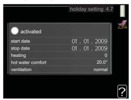
To reduce energy consumption during a holiday you can schedule a reduction in heating, ventilation and hot water temperature.
