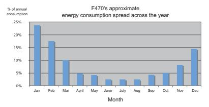
Increasing the indoor temperature one degree increases the energy consumption by approx. 5%.
