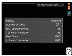
Information about the compressor's operating status and statistics can be obtained here. No changes can be made.
